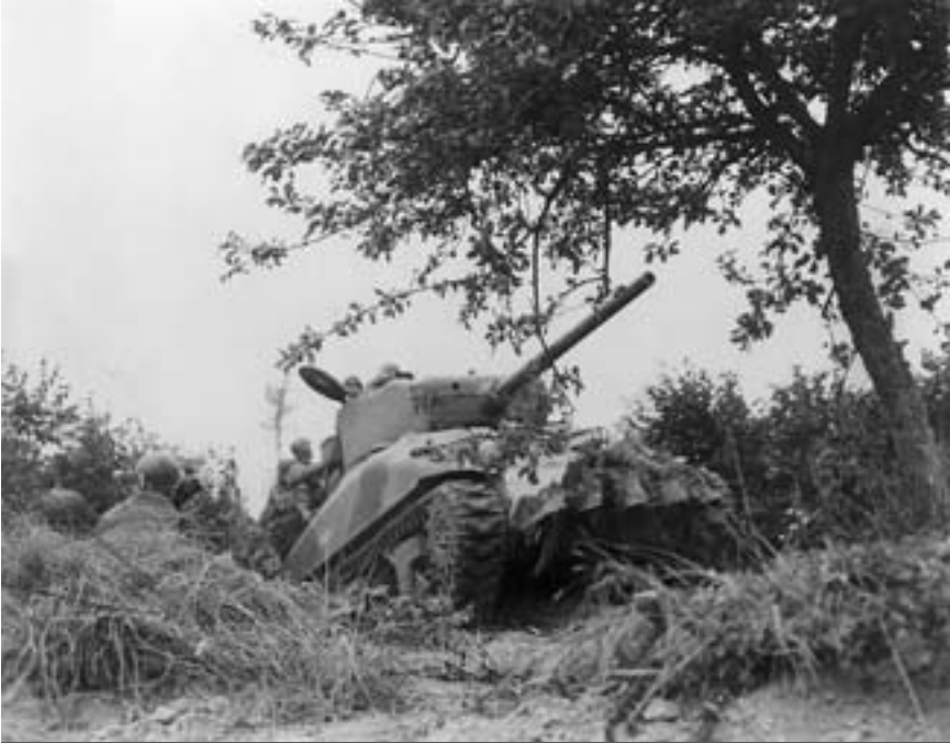
An M4 Sherman tank with hedgerow cutters (U.S. Army Armor & Cavalry Collection)
