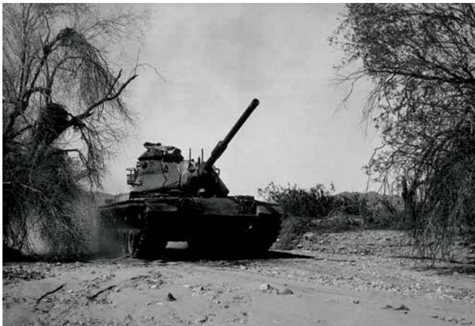
The M60A1 tank is tested on the dry-wash course at Yuma Proving Ground, Arizona. ( U.S. Army, National Archives Still Picture Branch )
