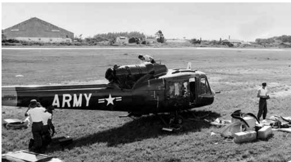
Maintenance personnel of the Utility Tactical Transport Helicopter Company assemble one of the newly arrived UH-1B helicopters at Tan Son Nhut, Vietnam. ( U.S. Army, National Archives Still Picture Branch )
