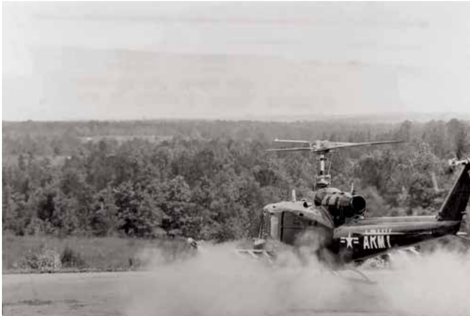
An HU-1 helicopter firing an SS11 missile (U.S. Army, National Archives Still Picture Branch)
