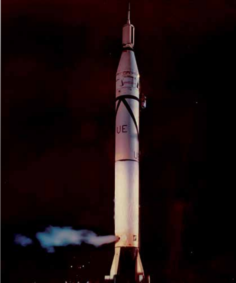
Explorer 1, boosted by the Army Ballistic Missile Agency's Jupiter-C missile, nears launching time from the agency's firing laboratory, located at the Florida Missile Test Range in Cape Canaveral, Florida. (U.S. Army, National Archives Still Picture Branch )
