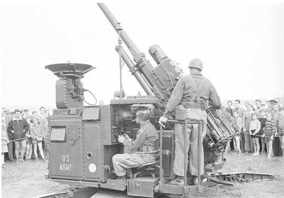
A radar-guided 75-mm. anti-aircraft gun, the U.S. Army's Skysweeper (Stadtarchiv Kiel, Schleswig-Holstein, Germany)
