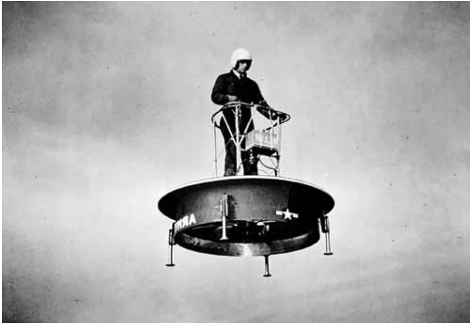
The Army's "flying platform," developed by Hiller Helicopters Inc., 1956 ( U.S. Army, National Archives Still Picture Branch )
