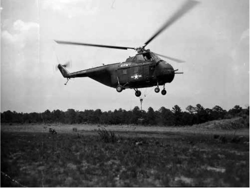
An H-19 Chickasaw carrying an external load, 19 July 1962 (U.S. Army, National Archives Still Picture Branch)
