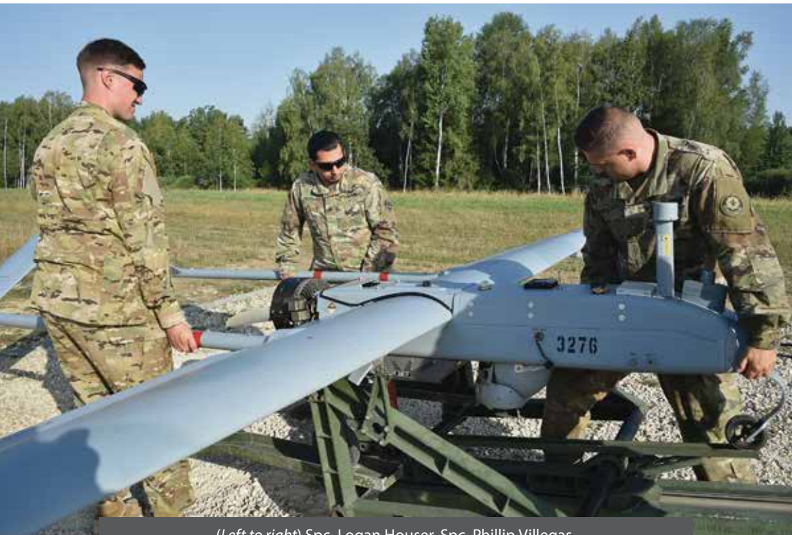
(Left to right) Spc. Logan Houser, Spc. Phillip Villegas, and Pfc. Ryan Longnecker mount a RQ-7B Shadow tactical unmanned aircraft system onto a hydraulic launcher at Balli UAS Airfield, Vilseck, Germany, 26 July 2019. (U.S. Army)
