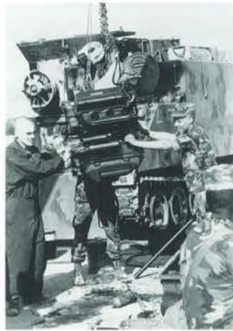
Engine overhaul at Ad Dammām
