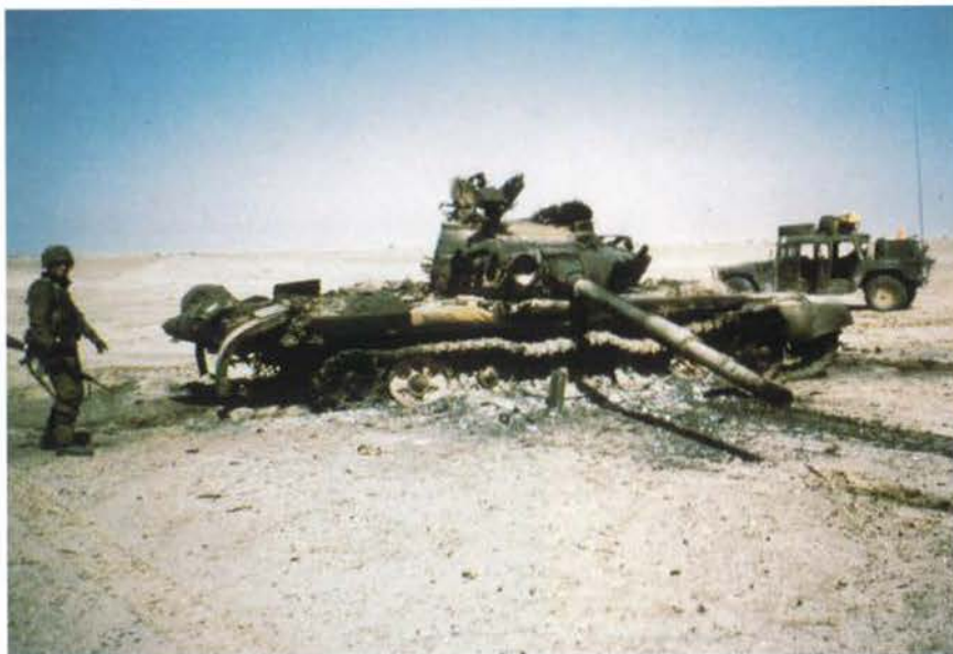
An Iraqi T-72 tank, penetrated and destroyed by two 120-mm. sabot rounds
