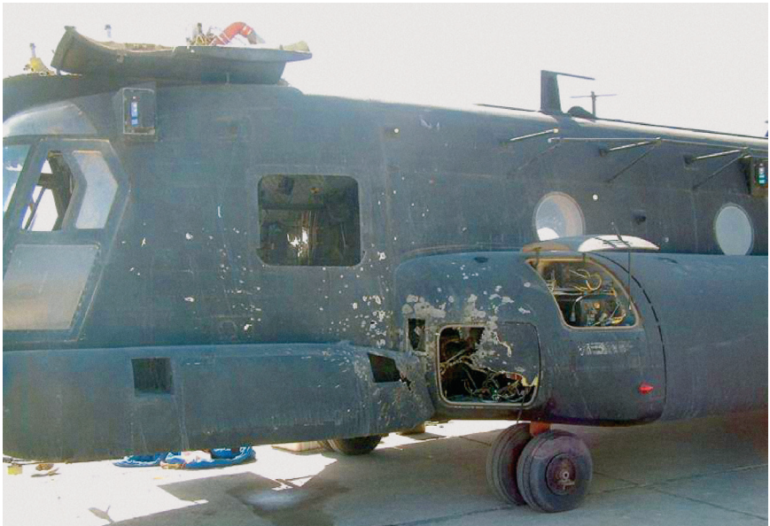
The MH-47 from the 160th Aviation (Special Operations) that attempted to insert MAKO-30 at the summit of Takur Ghar shows damage from a rocket-propelled grenade. (Courtesy of Duncan Sharp, former member of the Royal Air Force)
