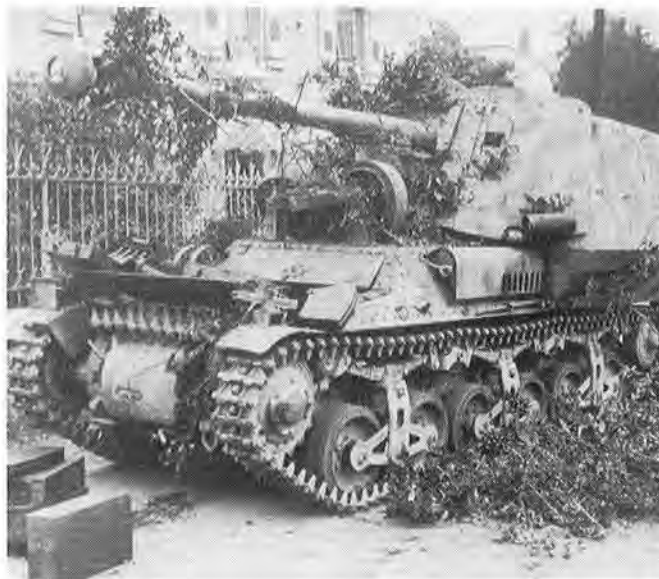
German 75mm, high velocity, self-propelled antitank gun
