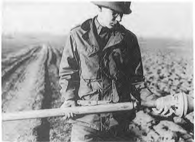
Panzerfaust 60 — one of four different models of a highly effective German recoilless antitank grenade launcher.
