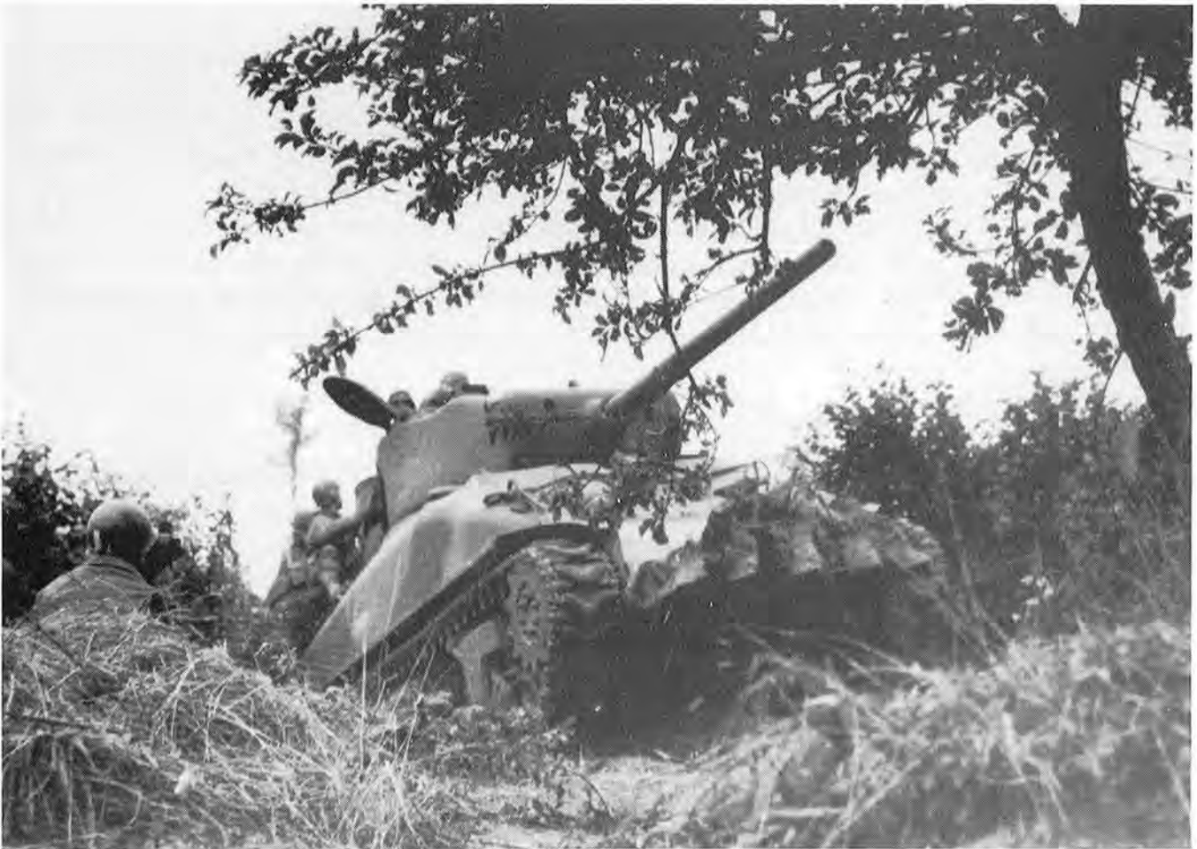
M4A1 Medium Tank equipped with a hedgerow cutter was used for breaking through hedgerows.
