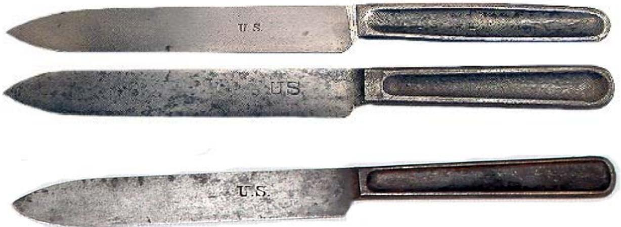
*Knives were made of cast iron in one piece with the blades polished and sharpened. The letters U.S. were marked on the blade.*
