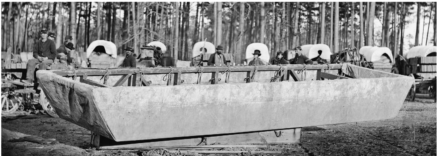
A canvas boat with its cover stretched over the frame and ready for deployment
