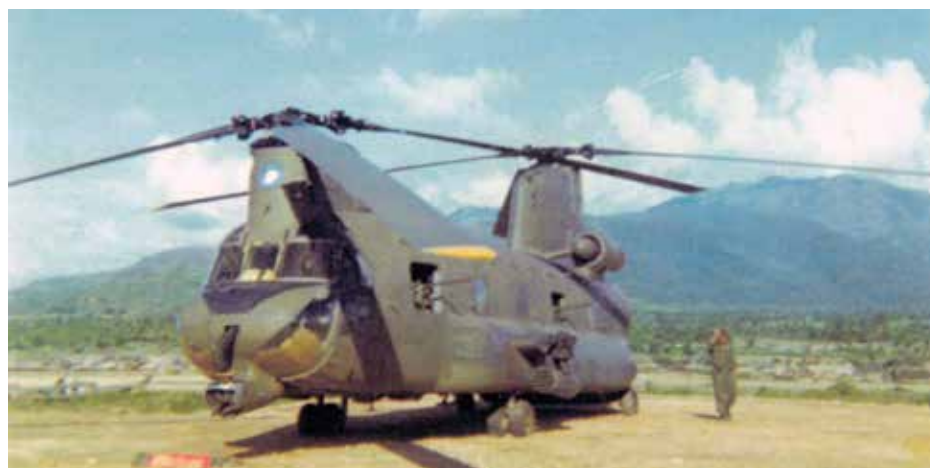
ACH-47A “Easy Money” after arrival at Vung Tau Air Base, Vietnam, ca. mid-1966. Note the loss of the glossy stateside paint job, though it is still possible to see portions of the roundel under the rapidly applied matte paint job for its field testing in Vietnam. Tedesco Collection, U.S. Army Aviation Museum
