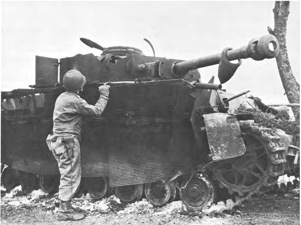
WRECKED GERMAN TANK SHOWING "BAZOOKA PANTS," a defense against rockets.
