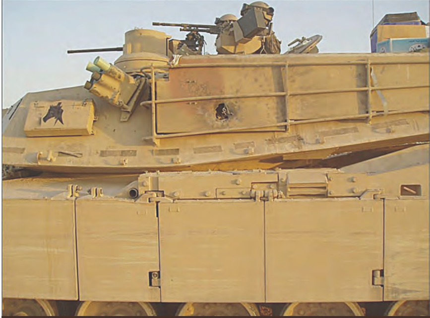
An RPG round hit Sergeant Beams' tank during the 21 August night raid on the parking garage. The resulting blaze in the sponson box cooked off machine-gun ammunition but otherwise inflicted no significant damage.
