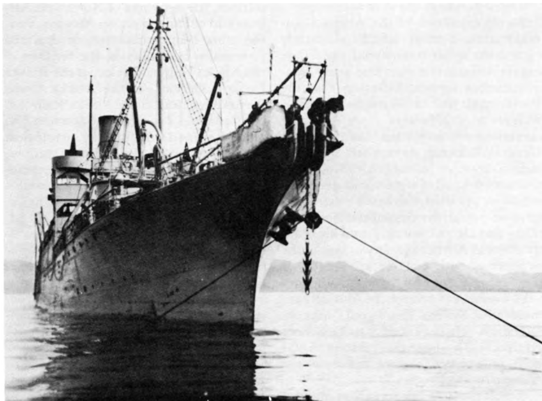
THE CABLE SHIP RESTORER . Note the cable grapple hanging from the bow of the ship.
