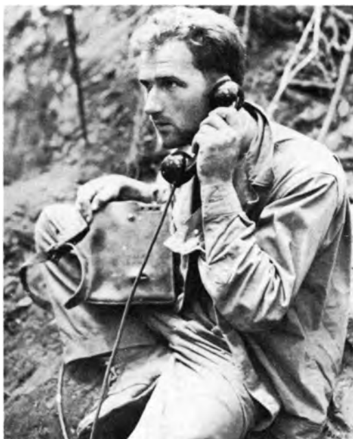
A BATTERY-POWERED TELEPHONE, the EE-8A. ( Photograph taken in 1943. )
