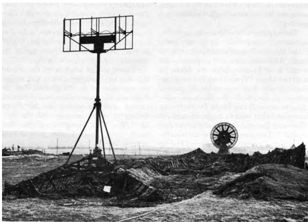
CAMOUFLAGED IFF EQUIPMENT of an American antiaircraft artillery group installed near Folkestone, England.
