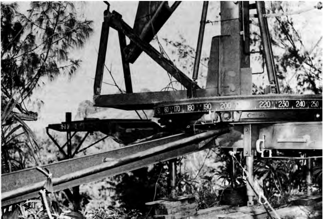
BASE OF SCR-270 RADAR, SHOWING AZIMUTH SCALE, VANUA LEVU, FIJI ISLANDS
