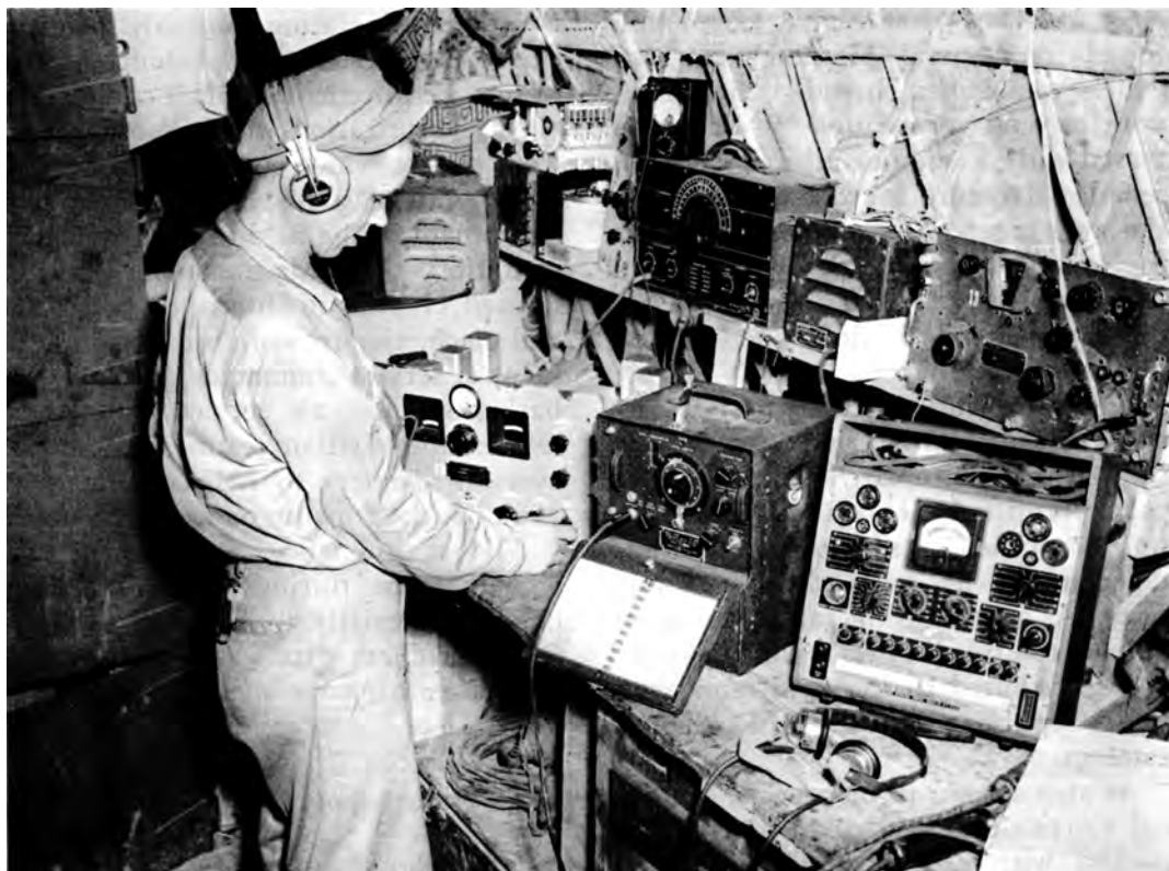
CHECKING THE FREQUENCY OF A BC-779-A RECEIVER at the signal repair section of General Stilwell's headquarters, Burma.
