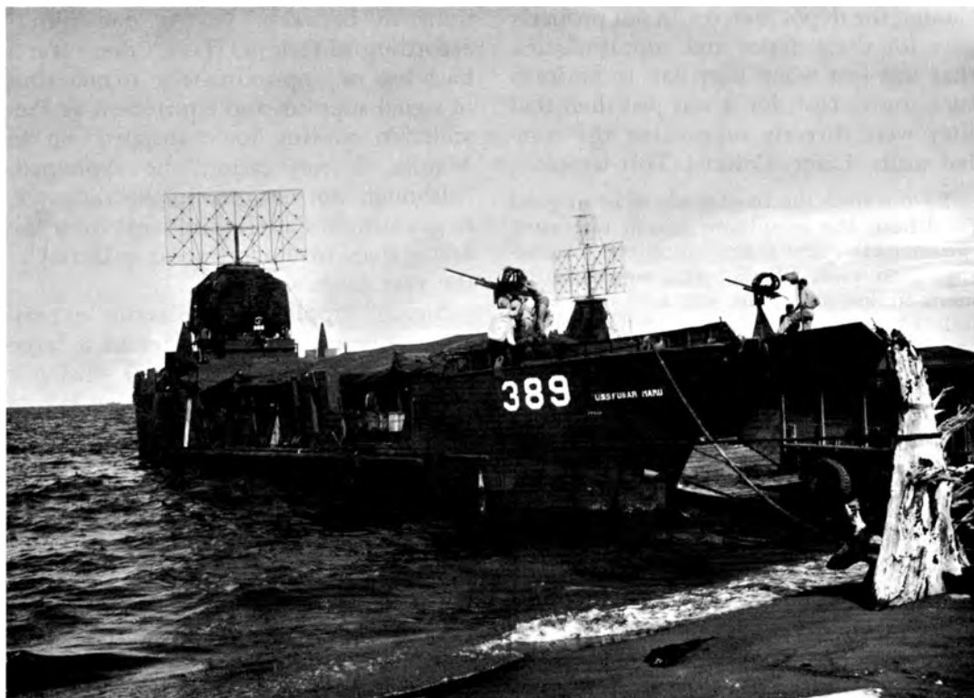
LW RADAR MOUNTED ON LST, NEW GUINEA
