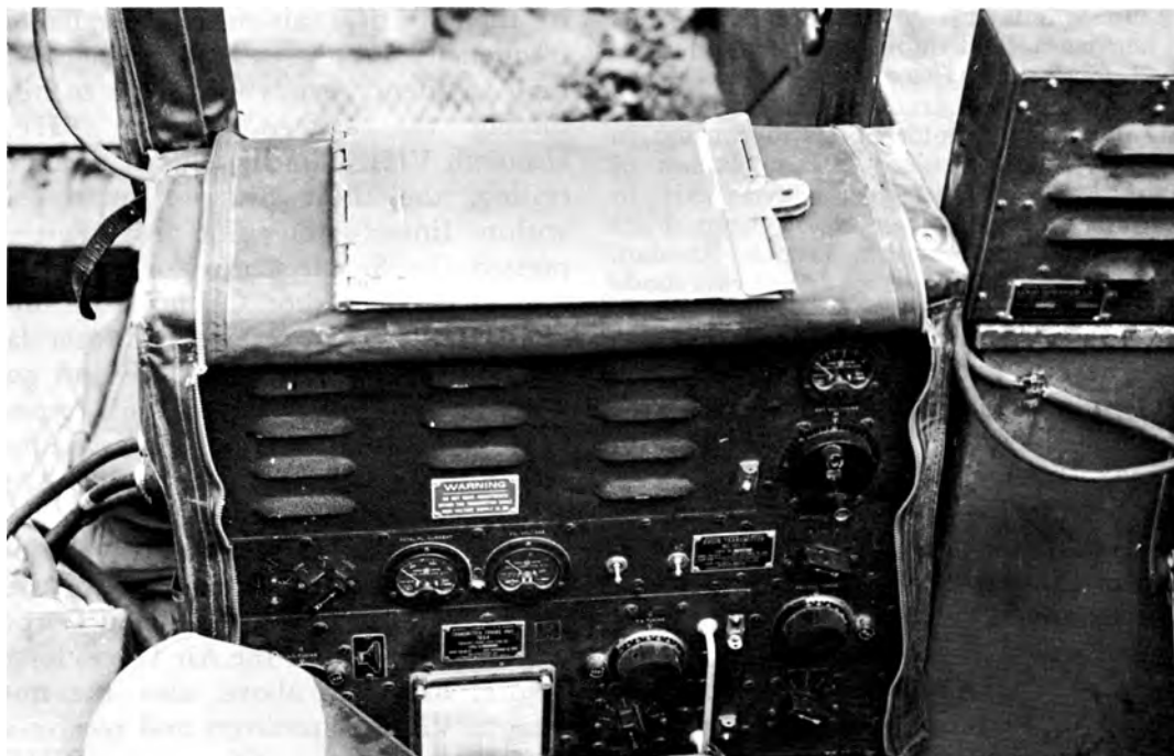
SCR-193 RECEIVING AND TRANSMITTING RADIO, MOUNTED IN A JEEP
