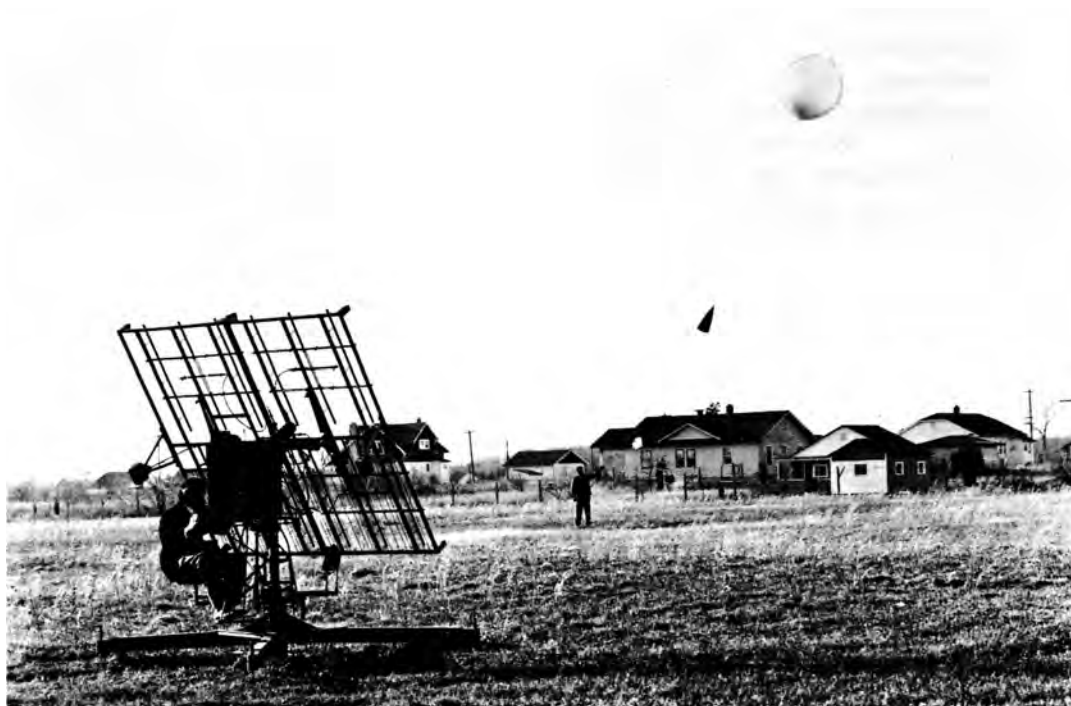
SCR-658 TRAINED ON RADIOSONDE AN/AMT-2 AT LAUNCHING
