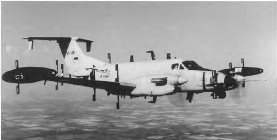
New systems such as the Guardrail Common Sensor mounted aboard the RC-12 platform enhanced the Army's electronic warfare and intelligence capabilities. (DA Photograph)
