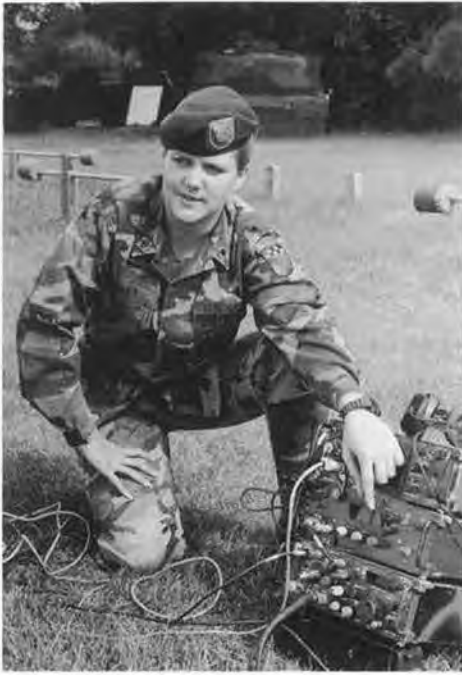
As a result of the Intelligence Organization and Stationing Study, the Army formed new Combat Electronic Warfare and Intelligence (CEWI) units to support its tactical formations. A soldier of the 519th Military Intelligence Battalion demonstrates a PRD-11 radio direction finder. (519th MI Battalion Photograph)
