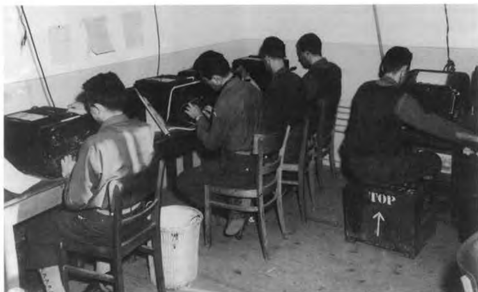
SSA guarded the security of U.S. Army communications, designing and producing electro mechanical cipher machines like the SIGABAs used in this communications center. (INSCOM)
