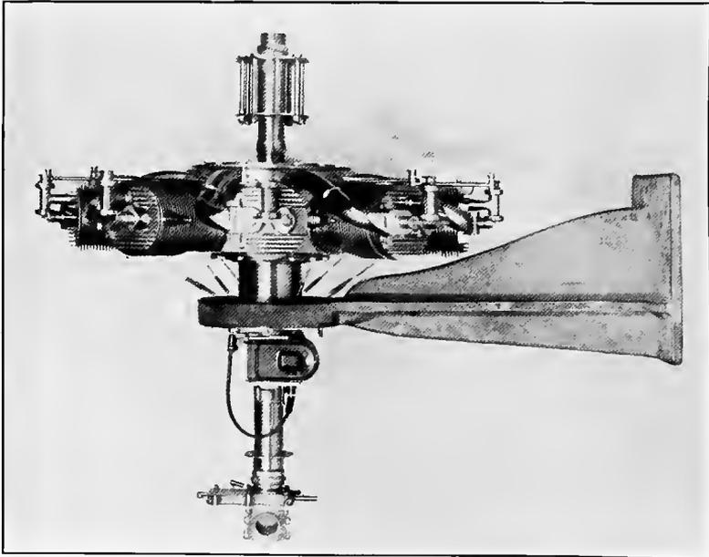
TWO VIEWS OF LE RHONE 80-HORSEPOWER ENGINE.
