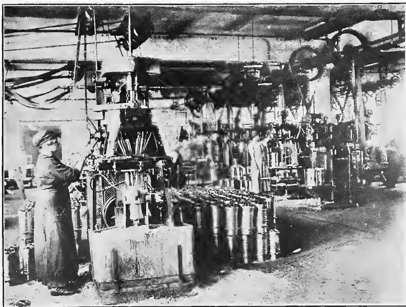
DRILLING CYLINDER FLANGES WITH MULTIPLE DRILL. PACKARD MOTOR CAR CO.
