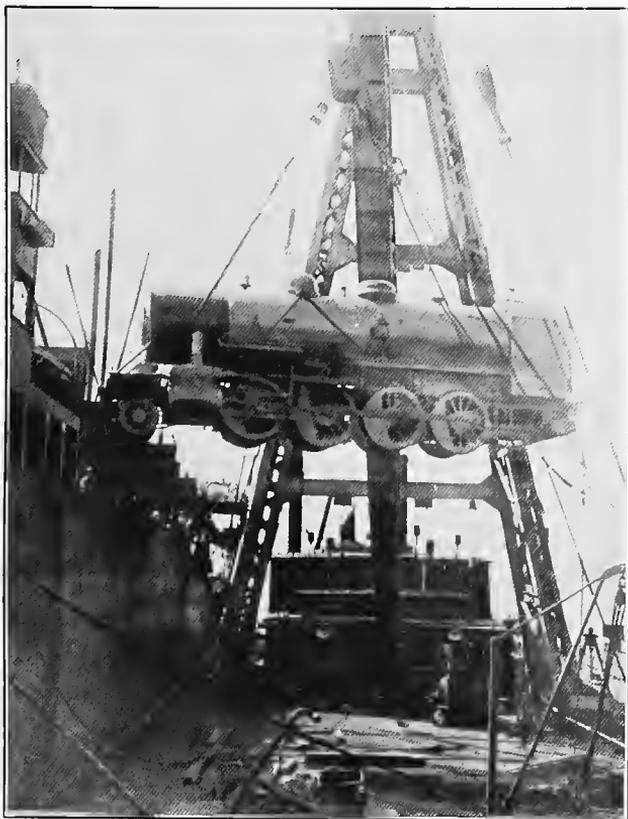
LOADING RAILWAY LOCOMOTIVES, COMPLETE, ABOARD SHIP.
