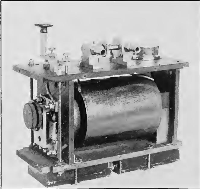
RADIO TELEGRAPH TRANSMITTING SET WITH CASE REMOVED.
