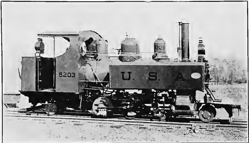
60-CENTIMETER GAUGE STEAM LOCOMOTIVE; TRACTIVE POWER, 6,225 POUNDS. CYLINDERS, 9 x 12, DRIVING WHEELS 23 $\frac{1}{2}$  INCHES, WHEEL BASE 5 FEET 10 INCHES; WEIGHT IN WORKING ORDER 34,500 POUNDS; CAPACITY: WATER 476 GALLONS, FUEL 1,700 POUNDS.
