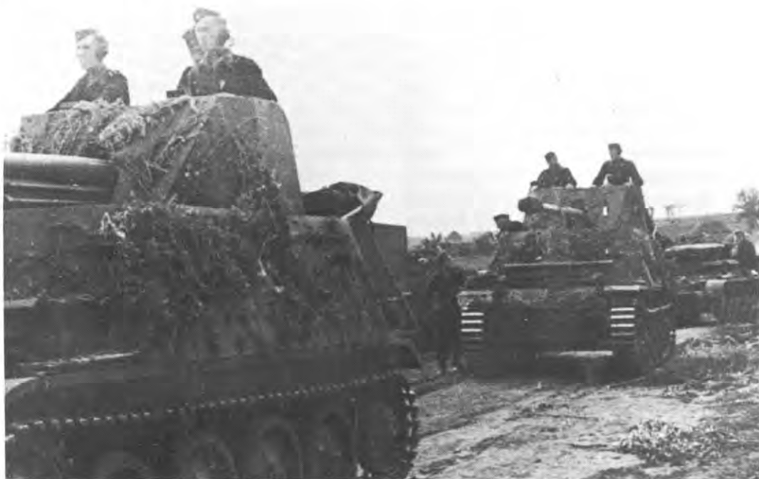
IMPROVISED MOBILITY: THE "MARDER" (MARTIN), Captured Soviet 76.2-mm. Antitank Gun on an Obsolete Tank Chassis
