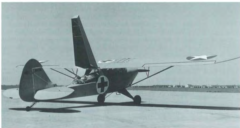
Douglas transport plane adapted for use as an air ambulance; below, Piper Cub modified for use as an air ambulance. Raised fuselage shows position of litter with patient.
