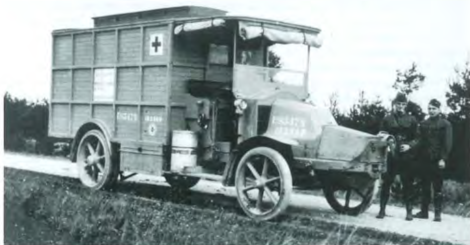
Renault truck outfitted with mobile x-ray equipment
