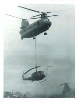
Damaged U.S. helicopter airlifted from Laos.
